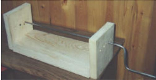
This instrument is used to wind coils. You drill a hole in the rod, and stick a portion of wire into it and wind the wire until you have a spring:
